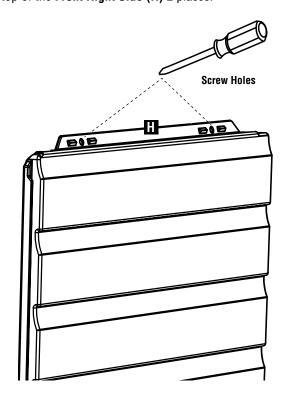
Drill a pilot hole (using 1/8" drill bit) in front lower corner at location indicated by screw target.
